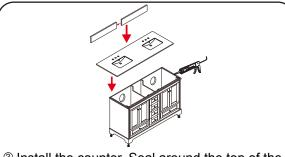
Install the counter. Seal around the top of the cabinet with clear silicone sealant. Do not over apply. Allow to dry 24 hours for proper curing.
