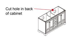
① Installer must cut appropriately sized hole in back of cabinet to accomodate existing placement of hot & cold wall valves & drains.
