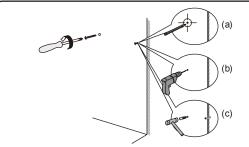
Install the mirror: a)use a pencil to mark the placement of the screw holes on the wall, b)drill holes, c)insert the plastic wall anchors.
