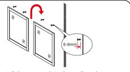
⑤ Install the screws into the wall anchors, leaving enough of the screw exposed to hang the mirror - approx 1/4" - 1/2".
