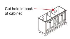
Installer must cut appropriately sized hole in back of cabinet to accommodate existing placement of hot & cold wall valves & drains.
