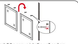
⑤ Install the screws into the wall anchors, leaving enough of the screw exposed to hang the mirror - approx 1/4" - 1/2".
