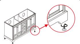
② Adjust the adjustable feet according to the floor.
