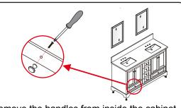
® Remove the handles from inside the cabinet doors and drawers and reinstall on the outside. Do not over tighten when reattaching.
