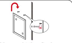
⑤ Install the screws into the wall anchors, leaving enough of the screw exposed to hang the mirror - approx 1/4" - 1/2".
