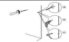
Install the mirror: a)use a pencil to mark the placement of the screw holes on the wall, b)drill holes, c)insert the plastic wall anchors.
