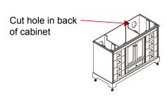
① Installer must cut appropriately sized hole in back of cabinet to accomodate existing placement of hot & cold wall valves & drains.
