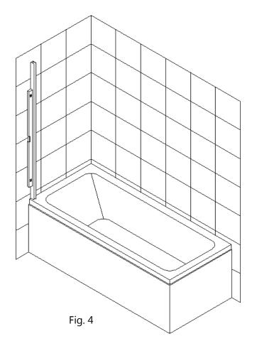
4. Mark the drill holes on the wall through the predrilled holes in the Wall profile (01). Now drill holes in the wall using a Ø5/16 drill bit and insert the Wall anchors (05). Apply silicone along the Wall profile and around the holes. Fasten the Wall profile to the wall with the Big head Screw ST4.2×40 (06).
