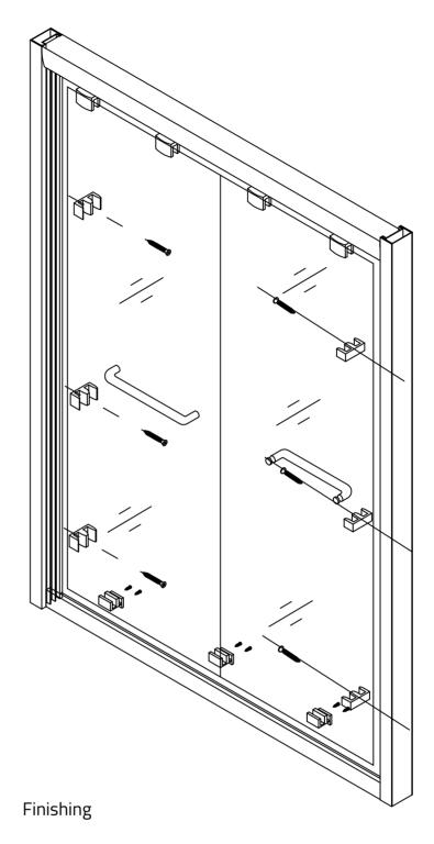
6. Install the stoppers (6). There are three on each side of the frame.
