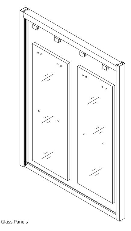
5. Now attached the glass panels (8) to the rollers. Fit two rollers to each glass panel.
