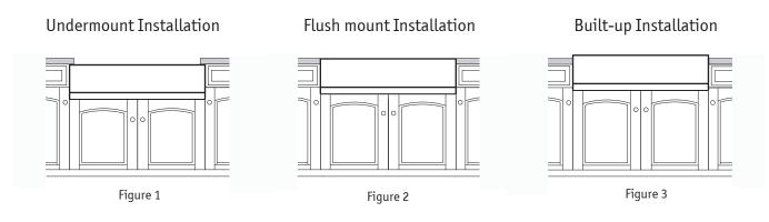
Caution: All installation types need to allow room for faucet installation. Ensure adequate clearance behind the sink for any faucet and backsplash, as well as full range of motion for faucet spouts and handles.
