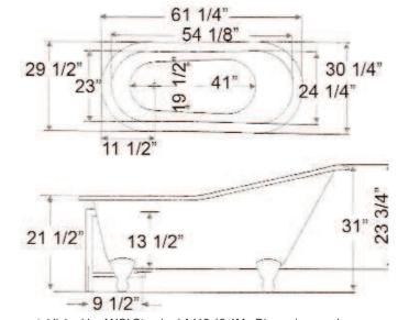
Dimensions of fixture are nominal and may vary within the range of tolerances established by ANSI Standard A112.19.1M. Dimensions and specifications subject to change without notice.
