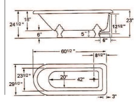
The following is recomended for ADTR60 tubs •Tub wall-mounted faucets •Double offset bath supplies: Part# 5576 •Leg tub drain: Part# 5599
