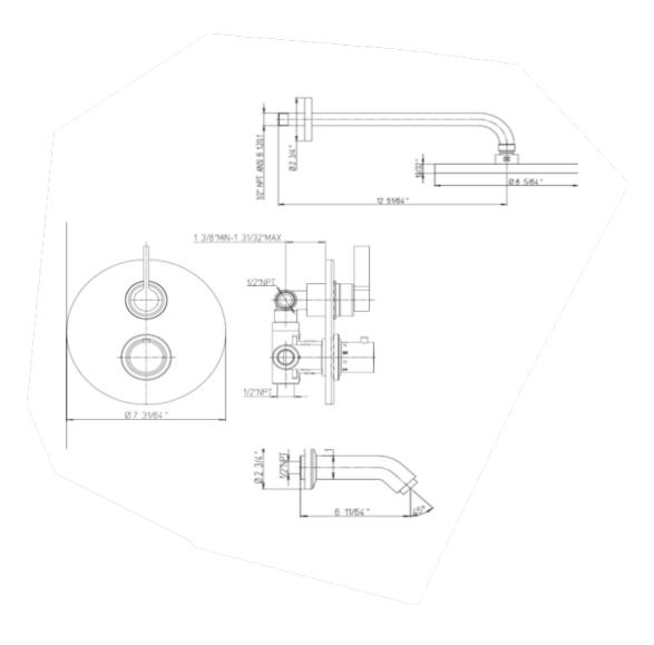
Elix thermostatic valve with 2way diverter volume control ½" inlet connections
