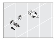
All models: Install the white plastic threaded sleeve to the hot and cold sides of the valve. Use a ruler to measure a point on the sleeve 3/8" from the surface of the finished wall. Mark the sleeve at that point. Cut the sleeve. Insert the inner sleeve.
