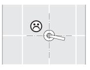
Remove the handle insert from the handle. Turn it slightly and reinsert it.
