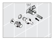
Use a ruler to measure to a point on the inner sleeve  $\frac{1}{2}$ " from the surface of the finished wall. Mark the inner sleeve at that point. Cut the inner sleeve. Push the handle into place.
