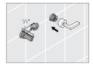
The handle should be parallel to the floor. If it is not, remove it.
