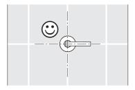
Remove the handle. Push the escutcheon over the outer sleeve. Place the handle over the valve. Turn the handle base clockwise, so that it threads onto the outer sleeve.
