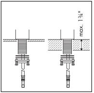
Hole size in deck: Minimum: 1 1/4" Maximum: 1 5/8" Operating pressure : max. 147 psi
