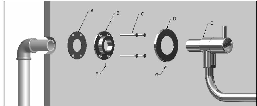
The adjustable flange allows for correct installation without the need for precise positioning of the internal pipe work. Therefore, the NPT connector should protrude from the wall / tile face 0 - 1/2".
