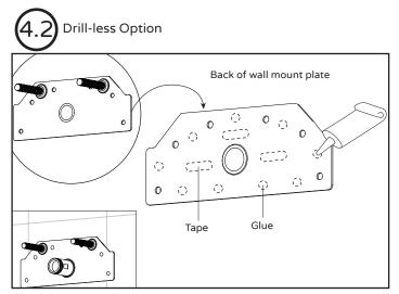
Apply glue (18) to wall mount plate(5) as indicated and add tape (included) to secure onto wall. Place wall mount plate (5) over holes drawn to make sure everything is leveled. Let glue (18)cure for 48 hours for complete result.
