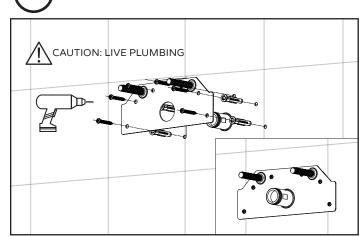
Drill hole previously marked and add anchors(7). Place wall mount plate(5) over the holes and secure with screws(8).
