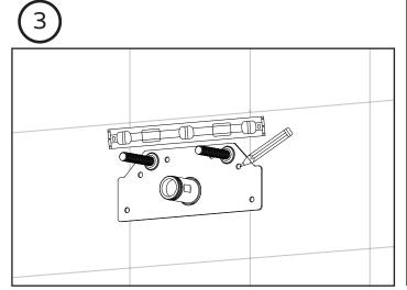
Place wall mount plate(5) over the inlet fitting(4) and make sure it is leveled. Mark holes with pencil.
