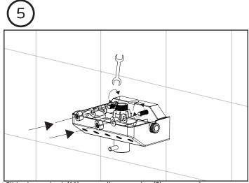
Slide shower body(11) over wall mount plate(5) screws and secure with nut(12).
