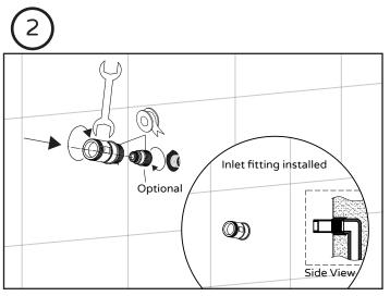
Apply plumber's tape on inlet fitting(4). If you need to use a nipple extension, be sure to also apply plumber's tape. Insert inlet fitting(4) onto existing water supply. Use wrench to secure.
